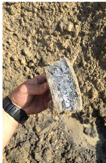
Cutting Steel: NX3600 charge used, 45mm severed
