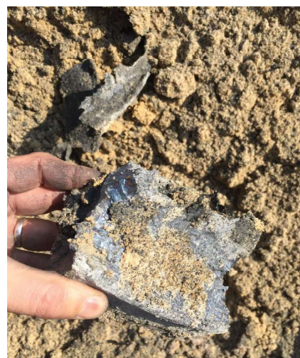
Cutting Steel: NX5600 charge used, 65mm severed
